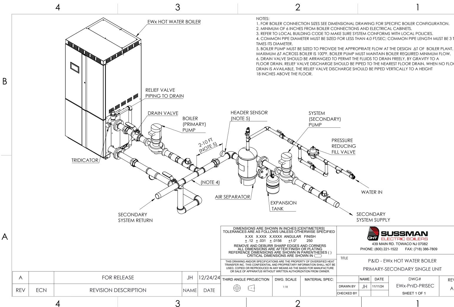
4. COMMON PIPE DIAMETER MUST BE SIZED FOR LESS THAN 4.0 FT/SEC; COMMON PIPE LENGTH MUST BE 3 TO 5
